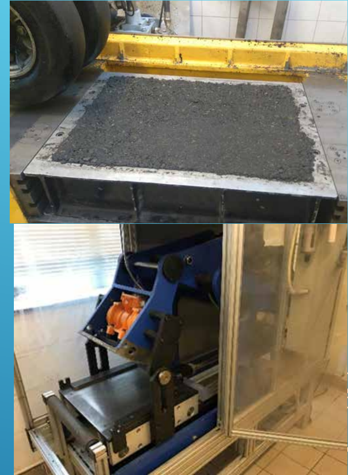
Simulation of compaction Compacted @ room temperature Grids available for characterization
