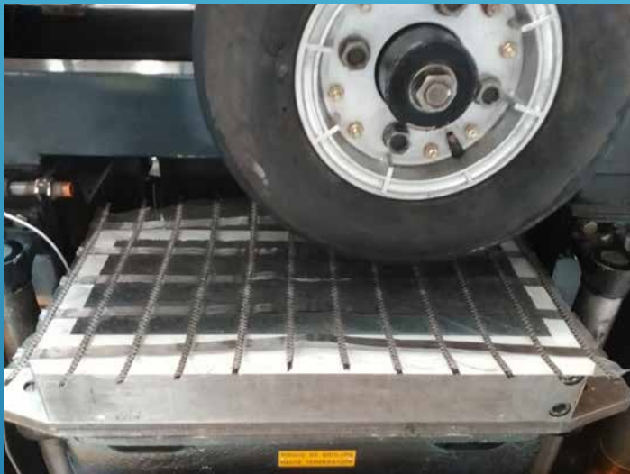
Effect of the traffic Grids over AC mix large rutting device 500 cycles
